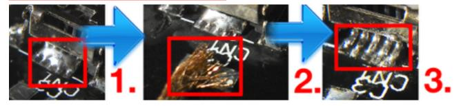
Fix the pads of the USB connector with **SOLDERING TIN** and generously apply **TIN** to the leads of the connector. Use **SOLDER WICK** like in (2) to free excessive **TIN** if your **SOLDER SUCKER** is not able to access the leads. Use the continuity tester of your **MULTIMETER** to check that there are no solder bridges between leads that are next to each other.
